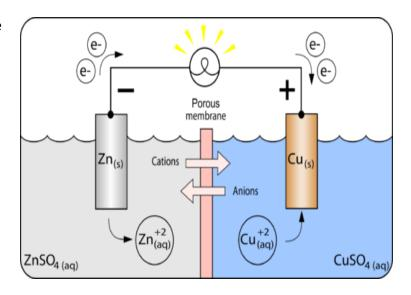
If the anode is connected to the cathode with a wire, electrons from the anode will flow towards the cathode. The electrons at the anode have \_\_\_\_\_\_\_, this is analogous to gravitational potential energy.
